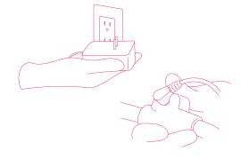
Connect the Control Head to the Power Hose and then re-insert the Light Stick. Be careful not to twist Control Head.
