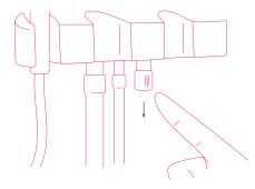
2 Attach hose connector to power vacuum hose and connect to HVE.
